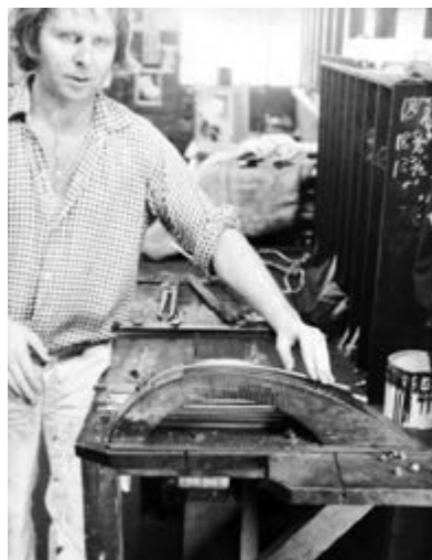
Making door forms
