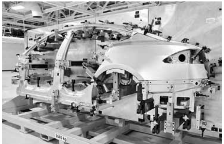
4 • left side body shell welded
