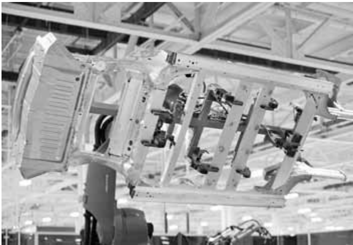
3 • stamped body pan with robot welder
