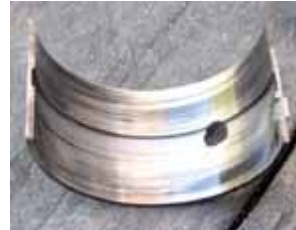
[above] bad center crank bearing
