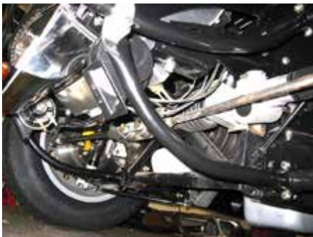
Triumph TR steering rack mounted on 1/2" steel plate
