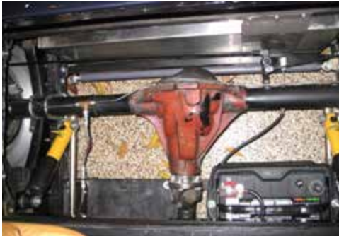
Rear Suspension shows track bars, panhard rod and tank safety plate
