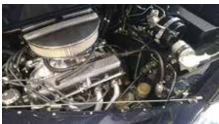
Engine area Dual Brake boosters and mystery bracket in front of left booster
