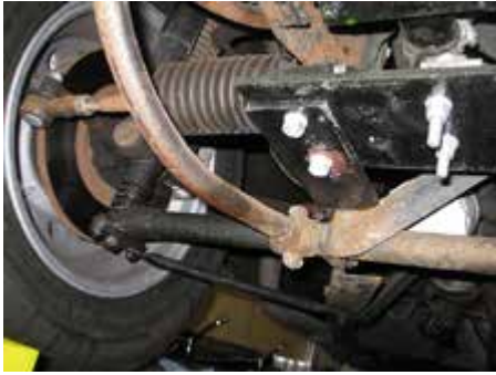
Triumph TR steering rack mounted on 1/2" steel plate
