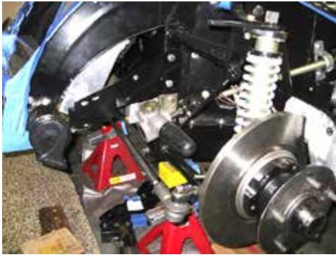
Front Suspension and new aluminum calipers
