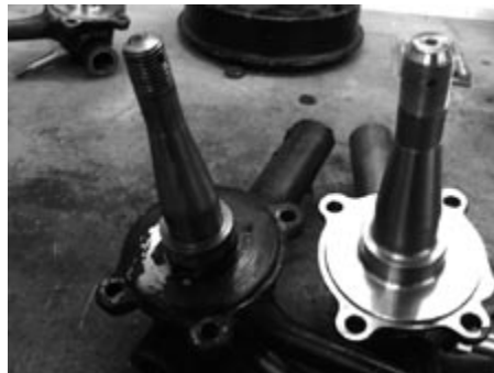
Axle 4: Comparison of original axle (left) to new competition stub axle.
