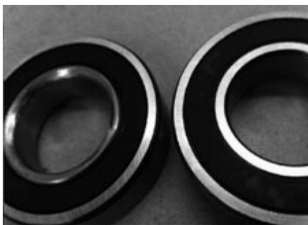
Axle 2: A 1/4" radius has been ground on one side of the inner bore of the bearing on the left to allow it to fit closely to the shoulder on the stub axle.
