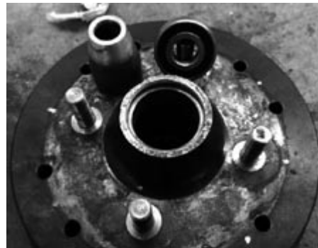
Axle 5: Drum/hub assembly after machine work. The bore has been opened up slightly to fit the new outer bearing and the aluminum spacer cone was repaired and bored out an additional 1/8" to fit over the new, larger stub axle.
