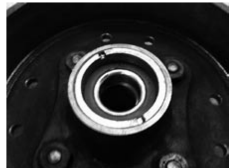
Axle 6: The original steel bearing retainer is used, but without a grease seal (note the bearing is the sealed type), which would now be too small to fit over larger competition stub axle. The screw-in retainer MUST remain in place and must be cotter-pinned for safety. Because the new bearing has a very slight different thickness, I re-drilled the cotter pin hole in the drum hub so that the retainer could be screwed in against the bearing and be secured in place. You can see the hollow conical aluminum spacer showing behind the inner race of the ball bearing.
